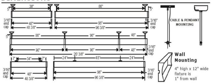
Patterns can be created using the corners shown. When fitting specific areas it is recommended that field measurements be supplied prior to fabrication
